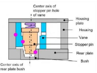
Beginning with certain 2008 models equipped with the R44, Honda began receiving complaints of a rattle on vehicle ignition. Investigation revealed that the pin in some R44s prematurely disengages from its seat in the bush, permitting the vane to bang violently within the housing, and produce a rattle. The "premature disengagement" that allows the vane to move freely only causes the rattle for a few seconds, because adequate oil pressure builds up
